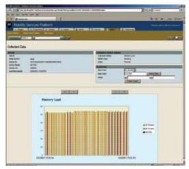
MSP3 offers the rich data collection and analysis capabilities required to simplify troubleshooting and enable rapid resolution of mobile device-related issues. A wide variety of metrics can be captured automatically over a period of time — either every 15 minutes or on the hour — and displayed in chart format for an instant at-a-glance assessment of device status.
